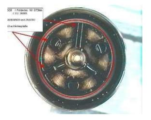
Sluggish Valve Piston Or Nozzle Needle
