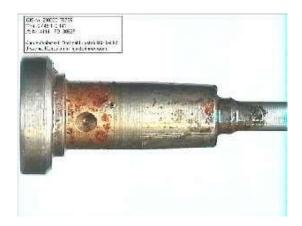
Sluggish Valve Piston Or Nozzle Needle
