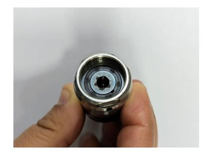
Internal Damage To Sensor Area
