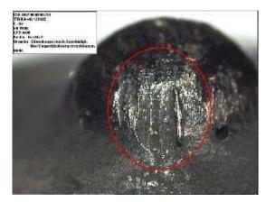
**Foreign Particle In Combustion Chamber**
