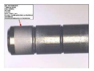
Poor, abrasive fuel (particles), Poor/inadequate filtration
