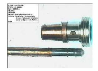
Sluggish Valve Piston Or Nozzle Needle
